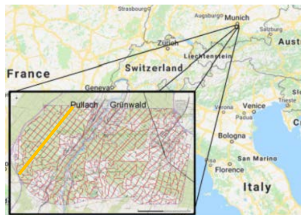
Figure 2: Location map of the 3D survey in Bavaria. (Red dots represent VP locations - Orange line is the XL2278 presented Figure 4).
