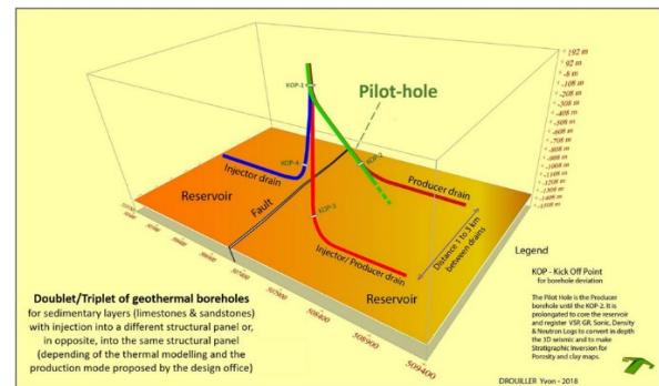
**Figure 4 - Example of architecture of boreholes with horizontal drains inside the reservoir which needs a better knowledge of the reservoir to manage (or not) the hydraulic connection. Where the design office will inject cold water? In a different structural panel or, in opposite, in the same structural panel? Faults location is needed.**
