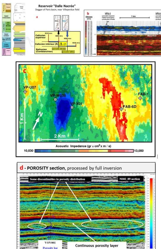
**Figure 5 - Reservoir "Dalle Nacrée": Variations of velocity and acoustic impedance explain POROSITY variations on Sonic log (a), 2D seismic profile (b) and 3D vibro-seismic horizon slice (c) – Variations of POROSITY on an inverted seismic section (d) - PICOREF project made in 1991-1993 by DHYCA to promote oil exploration in the Paris Basin [5- MOUGENOT D. et LAYOTTE P.C. - 1996]**
