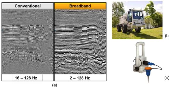
**Figure 6 - Onshore 3D seismic acquisition - Progress realized with the 6 octaves Broadband technique - 2-128 Hz (a), courtesy of PDO, single vibrator (b) and wireless geophones for use on urban sites (c), courtesy of Sercel**
