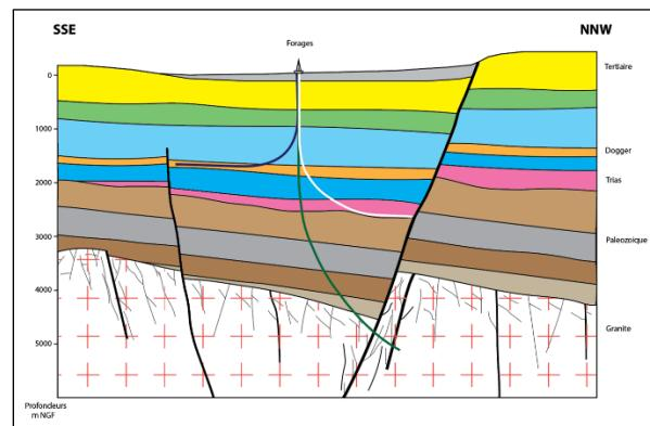
**Figure 13 – Project for geothermal exploitation of several superimposed aquifers: two stratified reservoirs and a fractured aquifer along a regional fault affecting the granitic basement, using the same 3D seismic dataset.**
