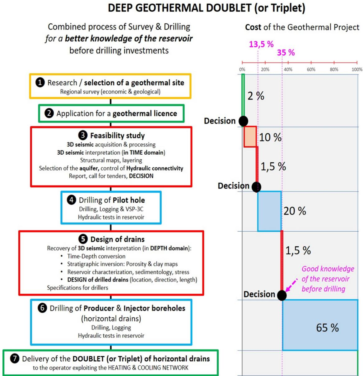
**Figure 11 - Combined Process for the survey of the objective aquifer (stratified or fractured) and design of geothermal doublets/triplets before drilling investments**
