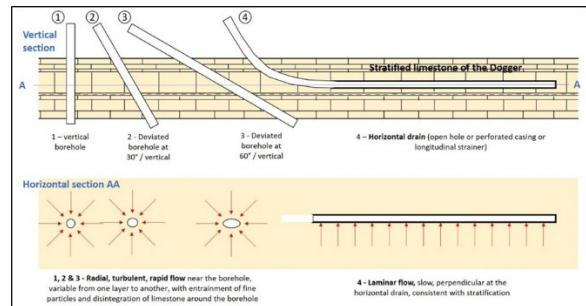
Figure 2 - Type of flow in the aquifer depending on the geometry of the borehole
