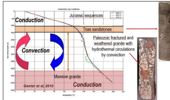
Figure 1 - Thermal profiles in boreholes at Soultz, in the upper Rhine graben [2 - GENTER & al., 2010]
