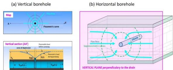
Figure 3 - Comparison of flows in a vertical borehole (a) and in a horizontal drain (b)
