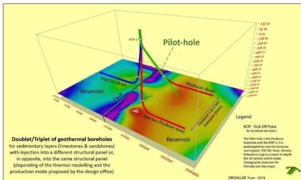
**Figure 12 - Example of a geothermal triplet with horizontal drains inside the reservoir. The porosity map (simulation here) characterizes the reservoir in each side of the fault. The better knowledge of the reservoir allows to inject cold water in a different structural panel. The third drain allows to inject or produce hot water, giving the operator both options depending on the season and the needs of the heating and cooling network.**
