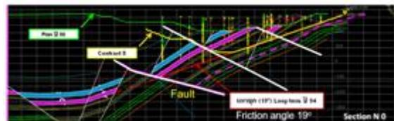
**Figure 4** Section of the pit - green curve is the current elevation profile - yellow curve is the future shape of the pit
