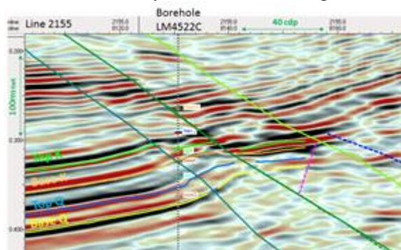
**Figure 7** Line 2155 with borehole LM4522C - K coal is 12m and Q coal is 24m thick.
