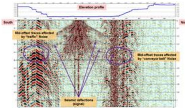
**Figure 5** Noise: traffic and conveyor belts.
