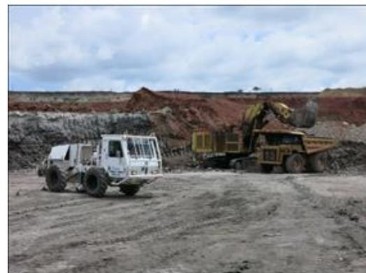
**Figure 6** Vibrator truck at Mae Moh mine
